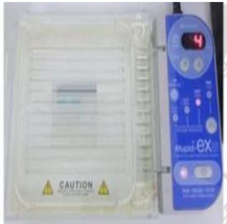
Gambar 5.5 Alat PCR set, (a) thermal cycler-merk thermo, (b) alat elektroforesis-merk mupid-Ex
