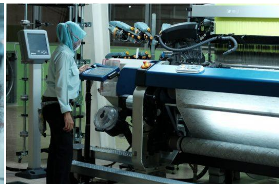
Gambar 4. Setting Alat Penenunan ( Air Jet Loom )
