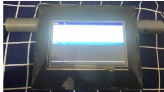
FIGURE 2. Ventilator Tester Display Ventilator Tester display with two PIP and PIF waveforms for validation
