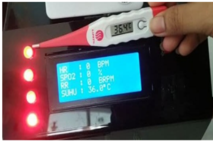
Fig. 4. The Display of Module Measurement Results with Body Temperature Value Comparison
