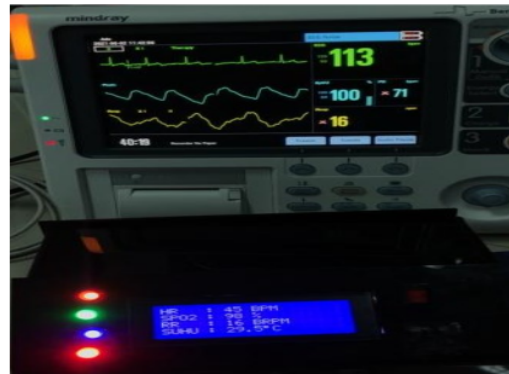
Fig. 3. The Display of Module Measurement Results with Comparison of respiratory rate values
