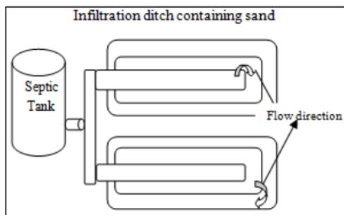
Figure 1 Design of Tripikon Infiltration
