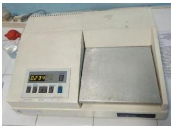
**Gambar 2.6** Alat Spektrofotometer UV – Vis *Single Beam*
