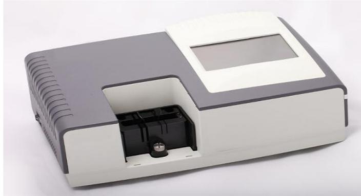
**Gambar 2.2** Alat Spektrofotometer *Ultra Violet-Visible* (Sawyer, 2019).
