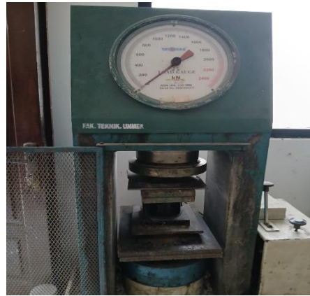
Gambar 8. Proses pengujian daya tekan paving block
